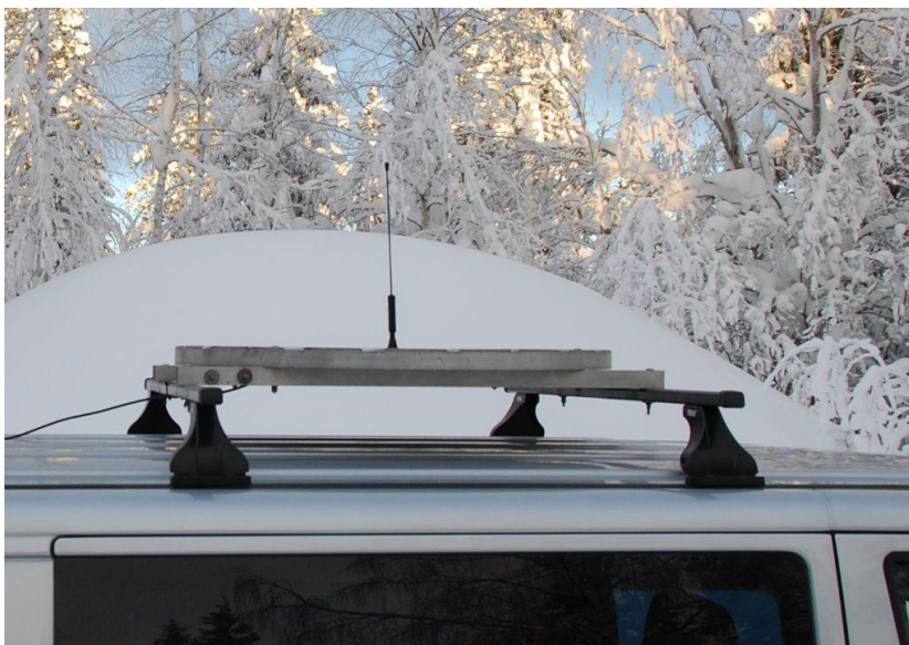
Figure 14. DAB antenna mounted on the roof of the vehicle.
