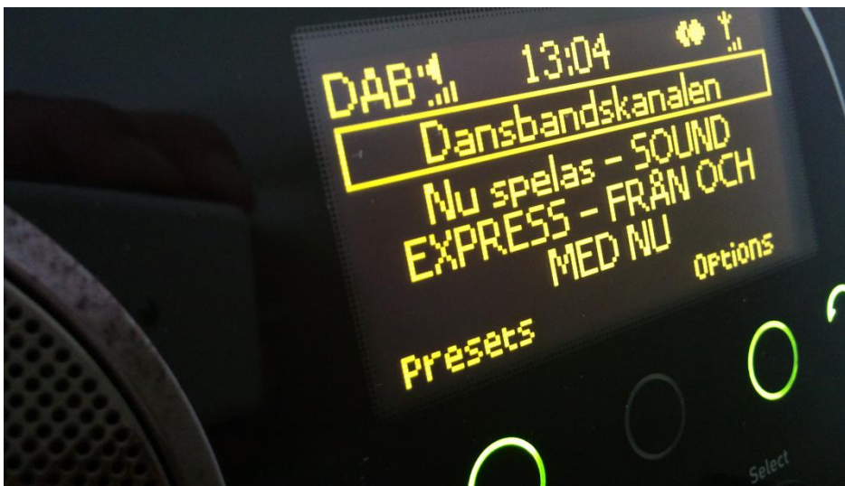
Figure 4. DLS dynamic text displaying “this song” and “next song” on a PURE EVOKE FLOW.
