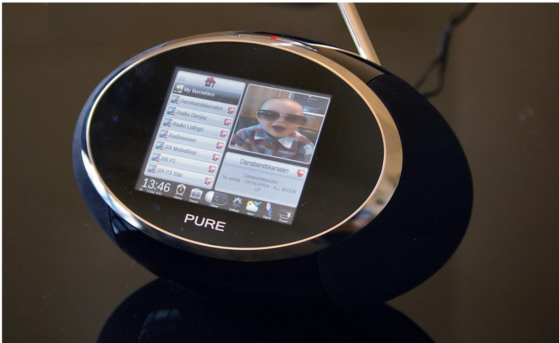
Figure 10. One of the participating radio stations broadcasts live from Sweden's many dancehalls. Teracom developed an application allowing their listeners to upload pictures to the digital radio platform, using their MMS enabled mobile phone. The pictures are being reviewed by the radio station and, if approved, published as a DAB+ slideshow along with the audio. The cost of sending the MMS, approx. 1 Euro, is charged to the listener's mobile phone bill and the revenues are split between mobile phone operator and the radio station.
